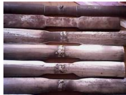
Fig. 3.4 Prepared samples for tensile tests
